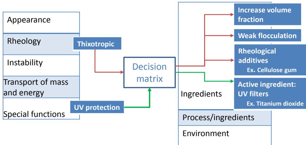
The first data base finds four possible solutions for the sub-problem. An active UV filter has to be used and thixotropic behavior can be enhanced by increasing volume fraction, enhancing weak flocculation or adding rheological modifiers.
