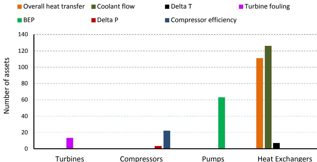
Figure 7: Existing PCM techniques for critical equipment at the Oxygen plant
