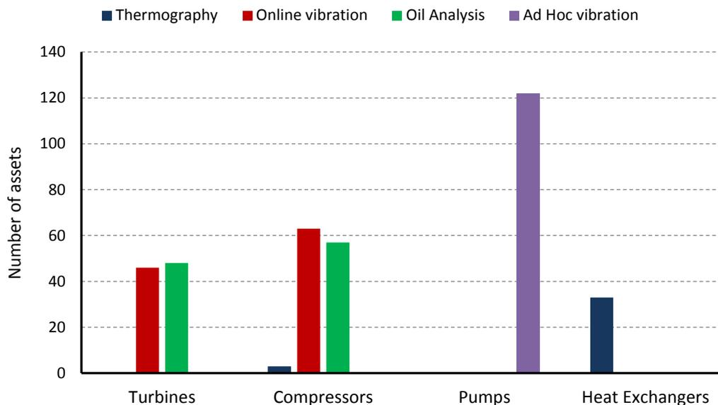
Figure 6: Existing CM techniques on critical equipment at the Oxygen plant
