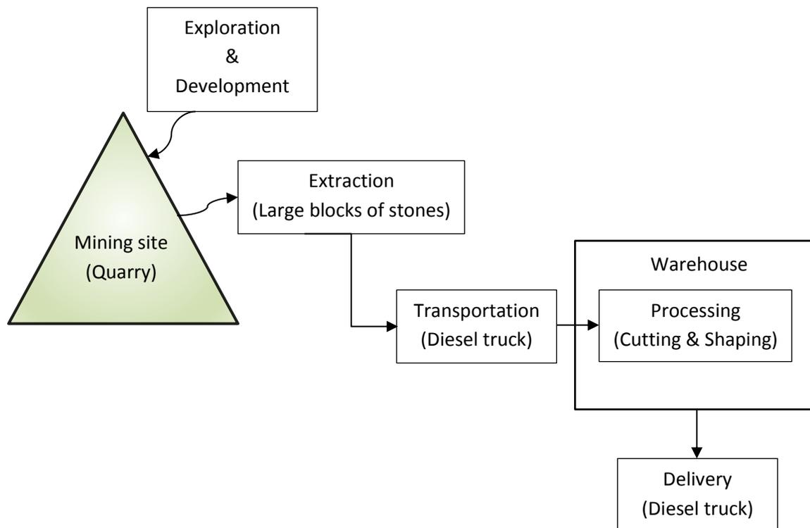
Figure 2: Artisanal sandstone mining process
