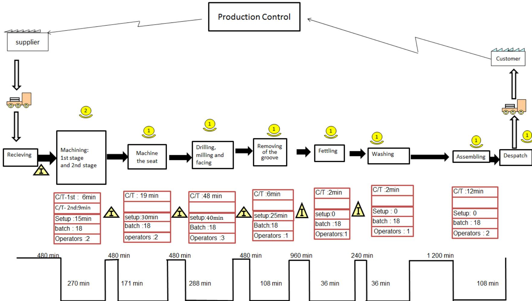
Figure 4: Future State Map - Paltech 100mm Butterfly Valve line
