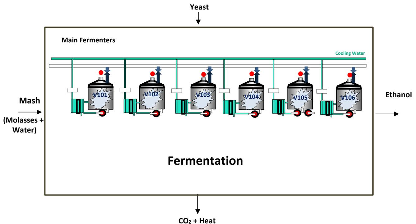
Fig. 6: The components in the Main Fermentation.
