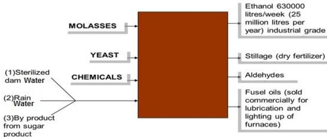
Fig. 4: The input and outputs noted during the pre-fermentation process.
