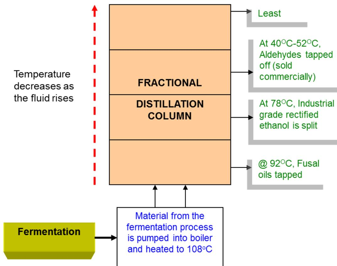
Fig. 7: The process and layout of the fractional distillation column
