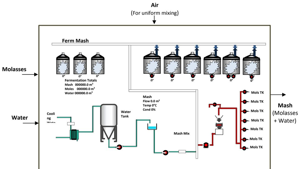
Fig. 5: The pre-fermentation process layout
