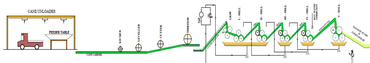
Figure 2: Sugar Cane Production Line Process Flow Diagram (Front End)
