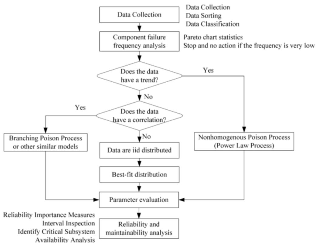
Figure 1: Reliability analysis process of a repairable system
