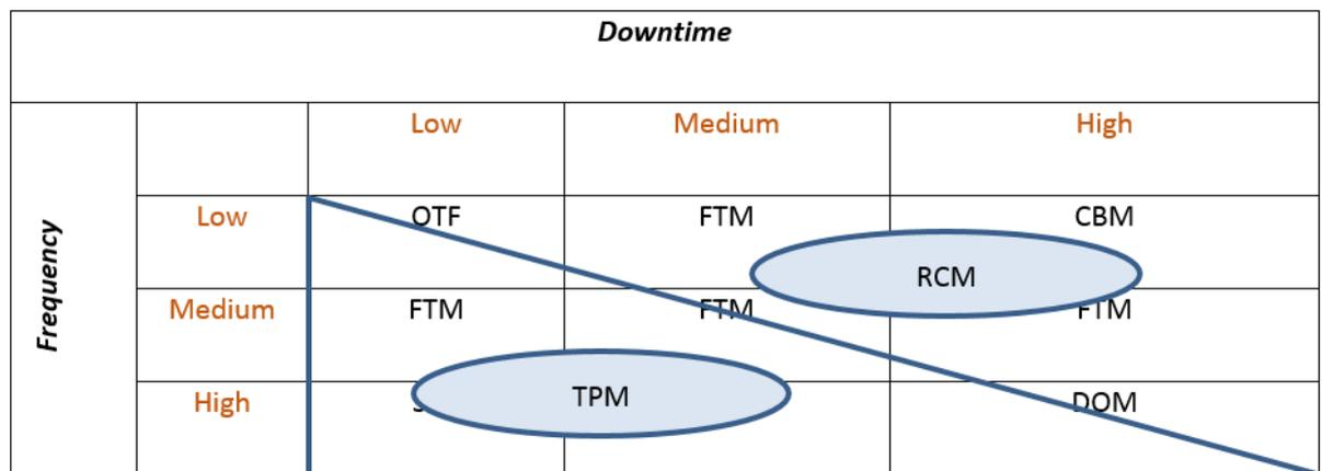
*Figure 3: Schematic classification diagram of management approaches to maintenance for a system of interest based on multiple decision criteria, here downtime and frequency of failure.*
